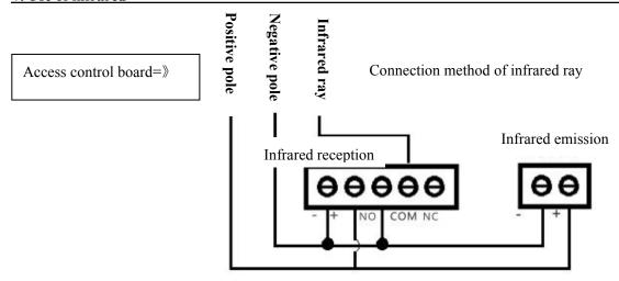
When the gate perform closing action, the infrared FSW is blocked, the gate stop and then bounce back to the open position to prevent pinching.
