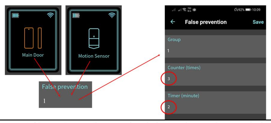
Without assigning to false prevention group, the sensors only need to be triggered once in order to trigger the alarm.
