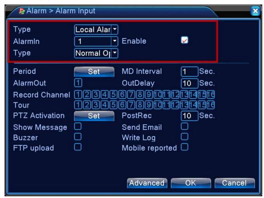
Alarm input is the same between hybrid mode & full digital mode, function enable, when it was set normal, only need to connect alarm sensor at alarm input port on local side, the alarm information is occurring, and will link to related setting functions at the same time
