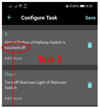
Condition become true **ONLY** when user turn off the Virtual Button of the Hallway Switch by physical **TOUCH**.
