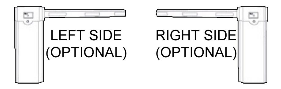
The left or right type is viewed by facing the door and the arm is at back of casing. For traffic rule following British way, we use mostly the Right side type.
